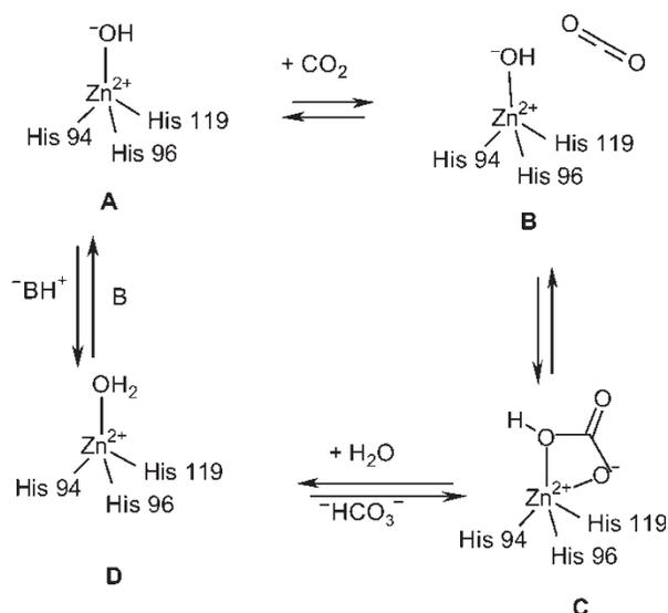
FIGURE 3 Schematic representation of the catalytic mechanism for the catalyzed  $\text{CO}_2$  hydration by  $\alpha$ -CAs.
