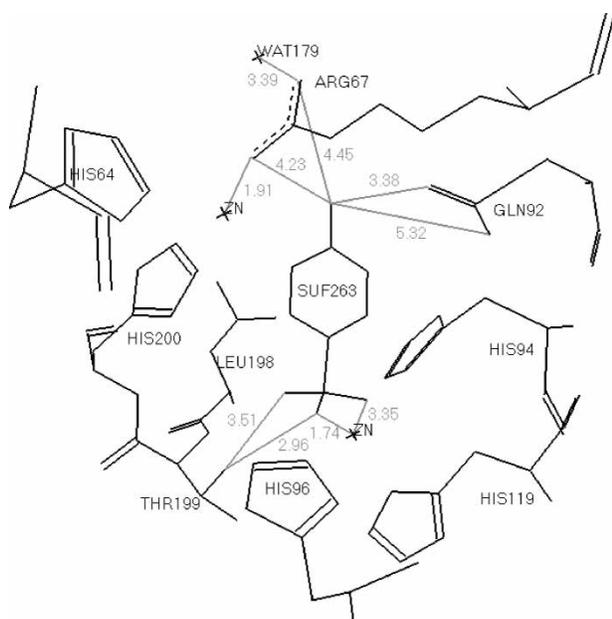
FIGURE 6 Model of sulfanilamide binding within the active site of the natural mutant, blood isozyme hCA I Michigan 1 containing two zinc ions (only molecule A shown), as determined by X-ray crystallography.<sup>18,19</sup>
